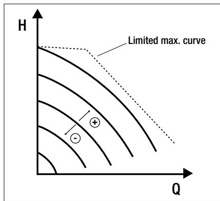
This control setting shows the curve of the circulator at constant speed. The operation curve is selected by setting the rotation speed on a percentage factor. Reaching 100% indicates the curve maximum. The speed of rotation may depend on power restriction and difference in pressure subject to model of circulator. The rotation speed can be set from the display or from an external signal 0-10V or PWM using the multifunction module.
