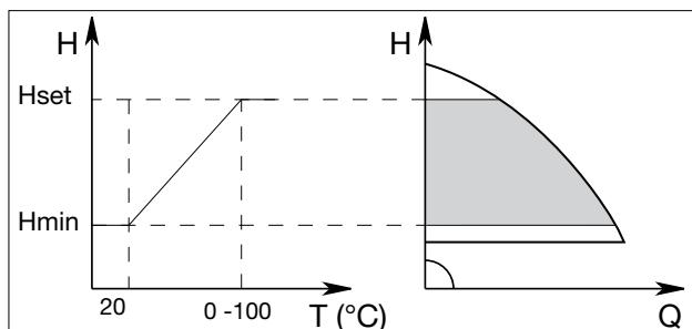
The circulator head set-point is reduced in accordance with the water temperature.
