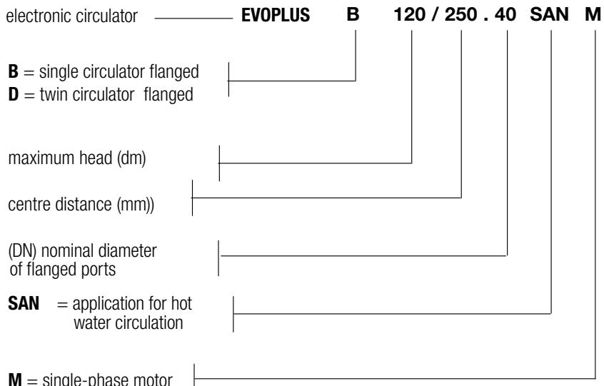
**Operating range:** 2 to 12 m<sup>3</sup>/h with head up to 11 meters;
