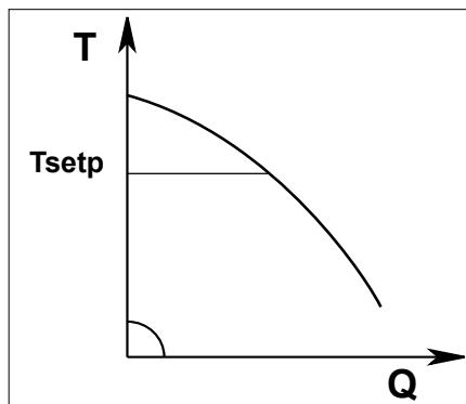
**$\Delta T_c$  control mode keeps the differential temperature of the pumped liquid constant, changing the flow rate to the user-settable value Tsetp.**
